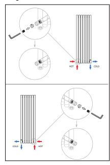
**IMAGE A:** The plug is screwed in on the left or right hand side, depending where the flow is entering.
