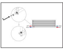
IMAGE B: When the product is to be mounted horizontally the threaded plug needs to be screwed into the left hand side of the radiator. This will force the water efficiently around the radiator whether the flow is coming from the left or the right hand side.
